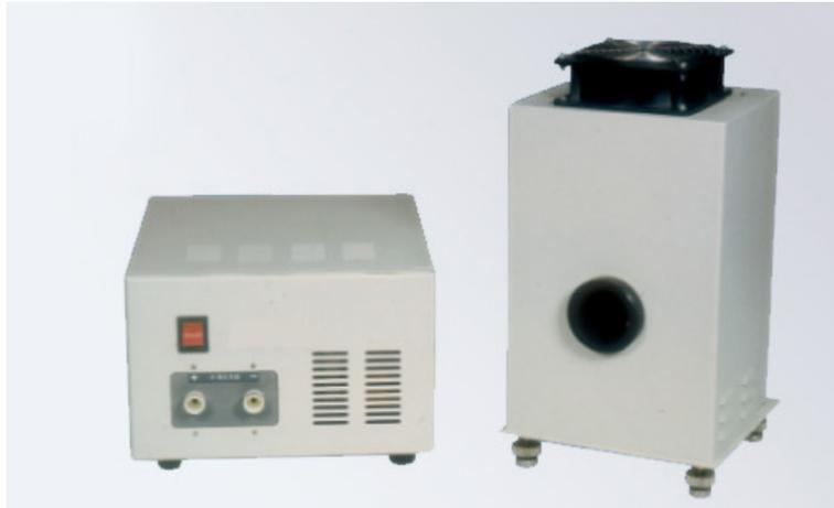
The lamp is a gas discharge light source and it is filled with high pressure xenon which can be excited by a high voltage and irradiate a strong and continuous spectra from ultraviolet to visible.
